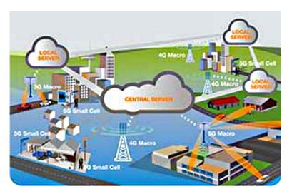
An illustration of 5G network architecture, showing 5G and 4G working together, with central and local servers providing faster content to users and low-latency applications.
