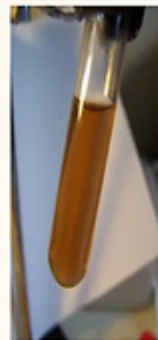
The oral sample after it has been subjected to a process of alkalinizing, heating and filtration. The sample is treated with sodium hydroxide ( NaOH ) in solution and heated to the boiling point. The solution is then filtered and produces the colored solution above. Please recall that the color of the ferric ion ( Fe^{3+} ) is usually yellowish to brownish and that the color of the ferrous ( Fe^{2+} ) ion is generally more greenish in color. This result of this process indicates that the ferric ( Fe^{3+} ) iron form is a candidate for further investigation in this qualitative analysis.
