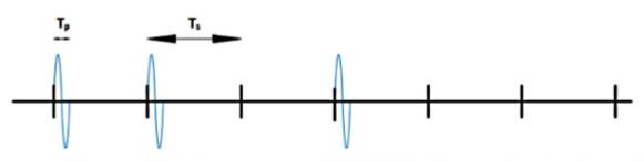
Transmitting the sequence "110100" with a pulse duration of 100 fs and symbol duration of 100 ps.
